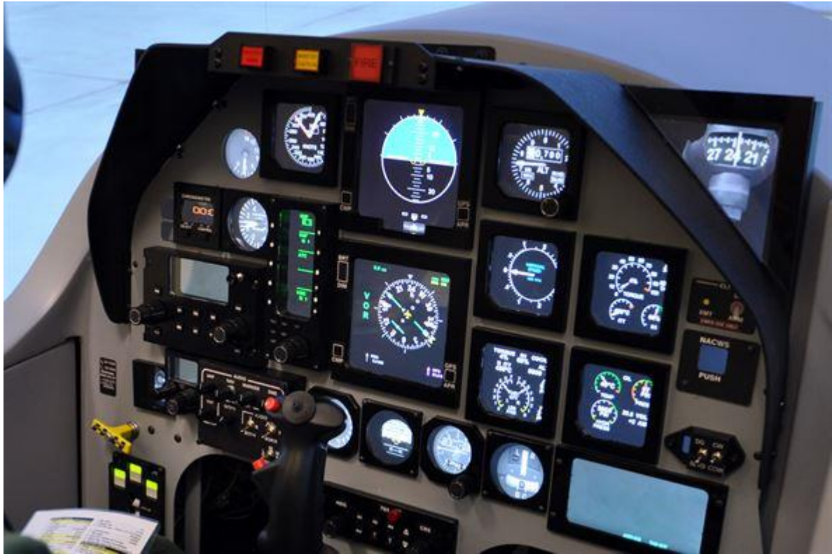
The new T-6 Texan II simulator instrument panel uses a single flat panel monitor and software to recreate the look and feel with digital displays and gauges. (U.S. Air Force photo/Staff Sgt. Clinton Atkins)
