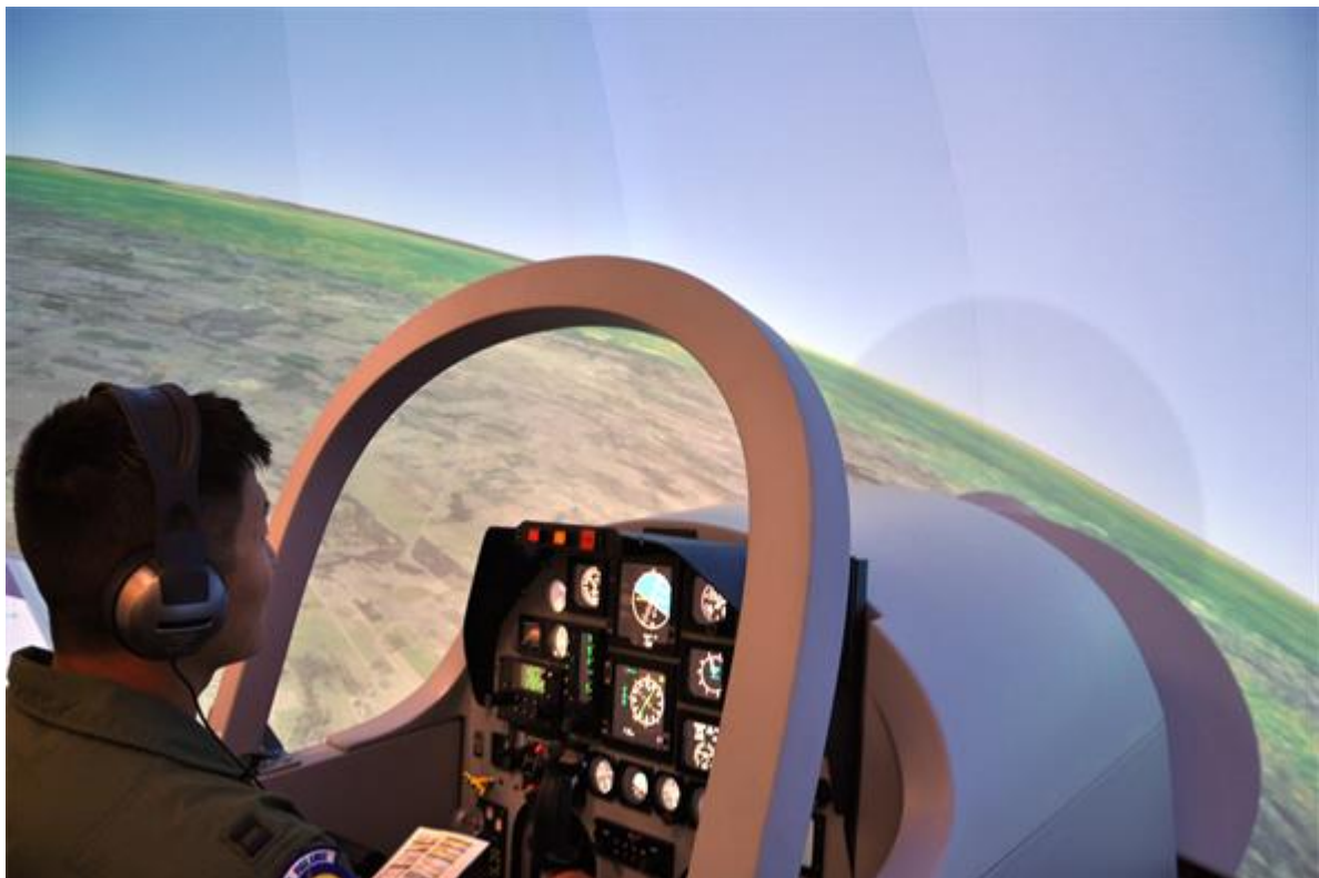
A student pilot enrolled in Undergraduate Remotely Piloted Aircraft Training at the 558th Flying Training Squadron, Joint Base San Antonio-Randolph, Texas, takes off in a new T-6 Texan II simulator July 10. The 558 FTS purchased 10 new simulators for $3
